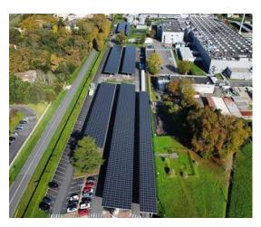
For its part, the Ambarès site (33) now has a similar installation with an installed solar capacity of 1.3 MWp, on more than 350 parking spaces also producing 1.5 GWh per year and avoiding 416 tonnes of CO<sub>2</sub> each year. This project also includes the anticipation of the installation of 70 charging stations for electric vehicles, to support sustainable mobility within the site.
